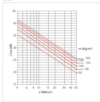
Figure C1 of the UNI EN 12354-2 standard, shows as, with an equal bulk for m' surface unit of the concrete,
